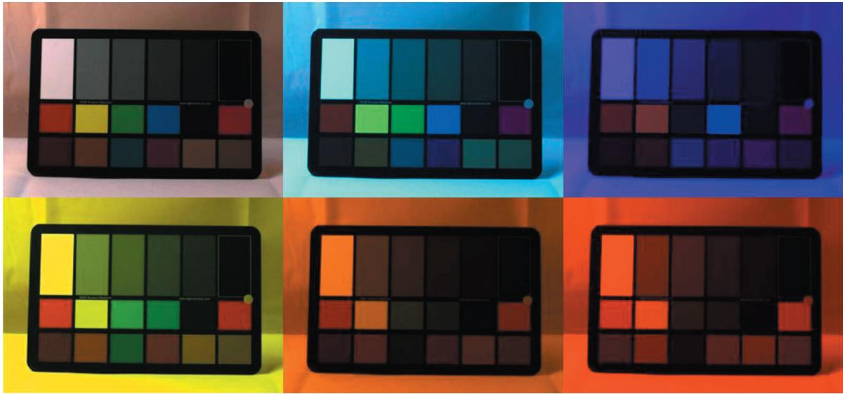
**Fig. 3.** Images of the same color table taken with the Canon 5D Mark III camera with fixed settings, but under different illumination conditions. This visually demonstrates the color metameristic phenomenon: the colors in different areas of the color table match or differ depending on the lighting. The images are reproduced from the MLSDCR (Multiple Light Source Dataset for Colour Research) (Smagina et al., 2020).
